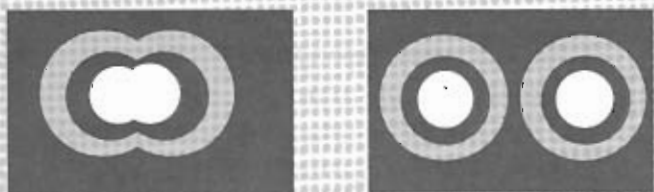
Figure 8.1 Diffraction limits our ability to distinguish two separate sources. In the first diagram the diffraction patterns have merged.
